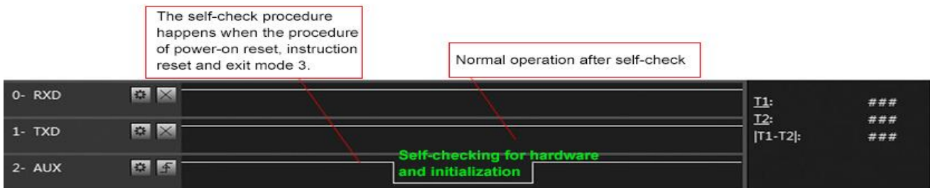
Timing Sequence Diagram of AUX when self-check
