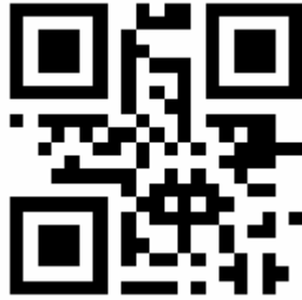
Figure I.2 — Final version 1-M symbol encoding 01234567
