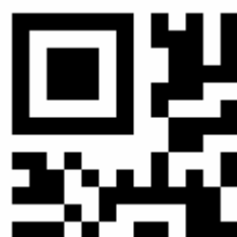
Figure I.4 — Final version M2-L symbol encoding 01234567
