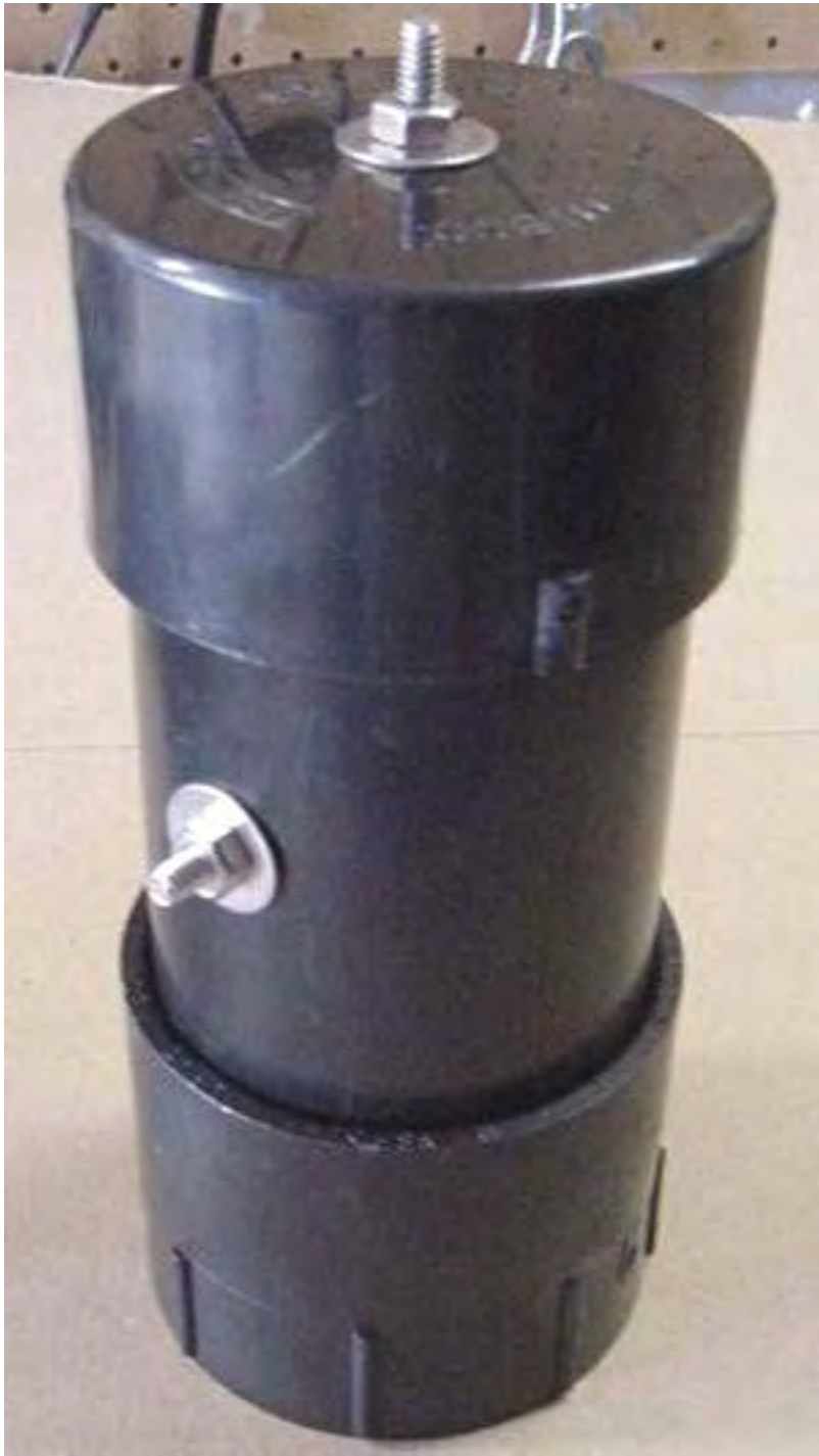
This is the finished e-cell shown here upside down. Assemble the unit using ABS glue.
