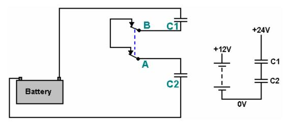
Here, the two charged capacitors are disconnected from the opposite supply rails and connected together to form a combined voltage of, in the case of a 12 volt battery, 24 volts connected across the 12 volt battery. This will cause a sudden inflow of current into the battery. However, before practically any capacitor current has flowed, the relay is operated again, repeating the sequence.
