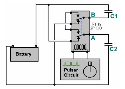
Here, the pulser circuit is set to give short, very sharp pulses to drive the relay cleanly. The relay has two changeover contacts "**A**" and "**B**". The operation is very simple. Initially, the capacitors "**C1**" and "**C2**" are charged up when the relay is in it's unpowered state and no current is flowing through the relay coil:
