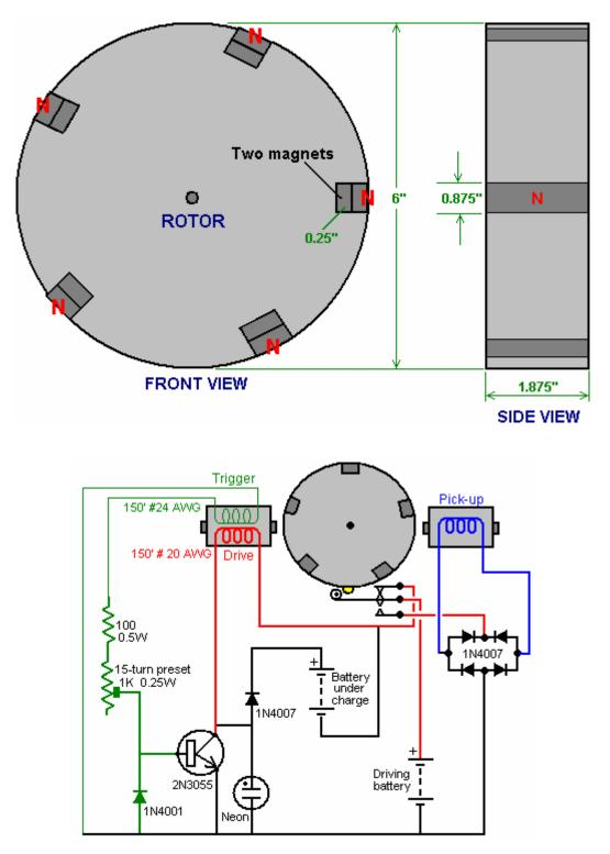
The rotor weighs about five pounds (2 Kg) and is very heavy for its size, because it is constructed from flooring laminate, and has a thickness of 1.875 inches (48 mm) to match the width of the magnets. There
