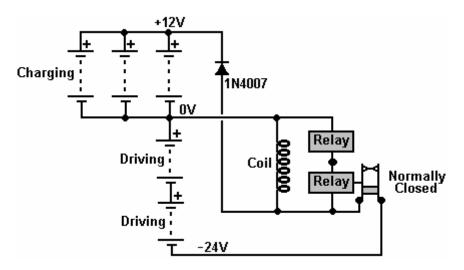
When using one of these relay charging systems you will find that quite a lot of noise is generated. This can be reduced quite easily with a little padding and it does have the advantage of indicating that the charging system is running correctly.
